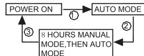
1. When the power is switched on, the sensor will enter into a "WARM-UP" period for about 1 minute and will then automatically change into "AUTO MODE".
