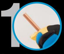
Firmly hold tubing at all times. Keep a safe distance between your hand and the tube's border.
