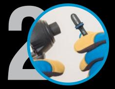
Choose bit size & attach it to the chuck or coupler. Fasten it well. Set power tool to MAX speed & torque if it is adjustable. Check power tool is not in hammer mode.
